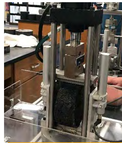
Image Source: FHWA Load Frame performing Ideal-CT
